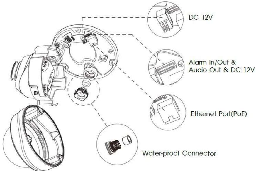
(AI) Motorized Pro Dome Network Camera multiple interface cable (Version D)
